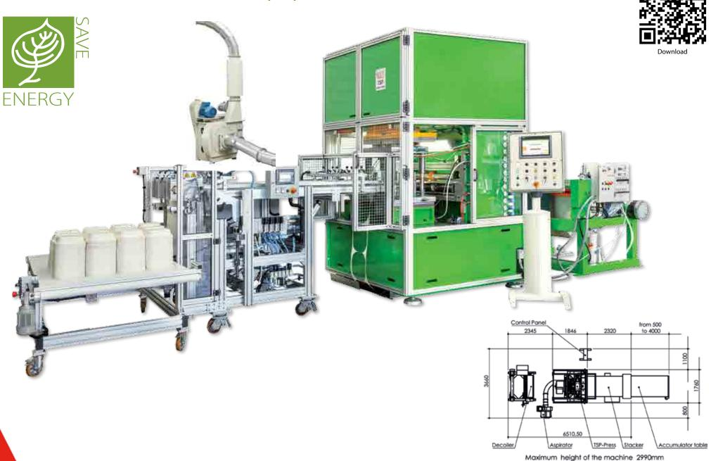
The new revolutionary TSP press has been designed and developed for the production of aluminium and paper food containers, dishes and trays. These products are obtained by blanking and forming of aluminum or paper which has been unwound from a coil.
